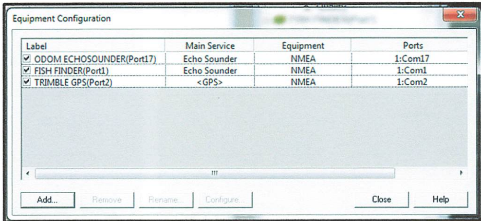
Gambar 3.7 Setting GPS, Hydrotrac - Odom Hydrographic Systems dan Fish Finder Garmin GPSMap 585 dalam software Hydropro 2.40
