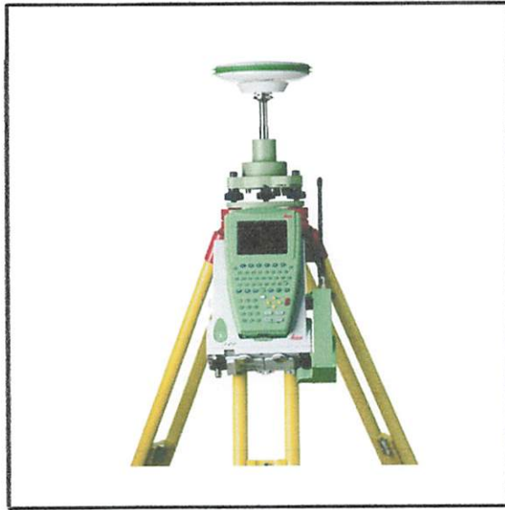
Gambar 2.7 Contoh Receiver GPS Tipe Geodetik (sumber www.esri.com )
