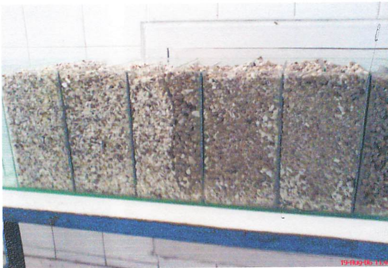
Gambar 8. Tampak depan Roughing Filter aliran horizontal
