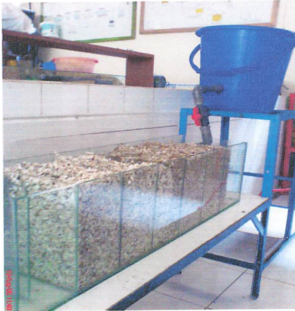
Gambar 7. Tampak samping alat Roughing Filter aliran horizontal
