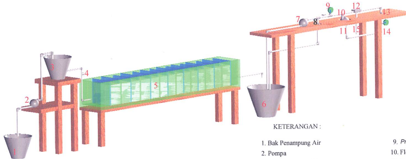
Gambar 3.2. Rangkaian alat Proses Pengolahan Pretreatment Roughing Filter aliran horizontal dan Treatment Membran Mikrofiltrasi Metode Crossflow
