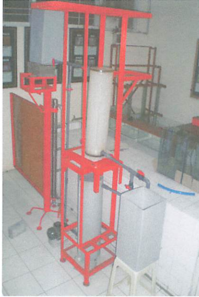
Gambar Rangkaian Dissolved Air Flotation (DAF) System Recycle
