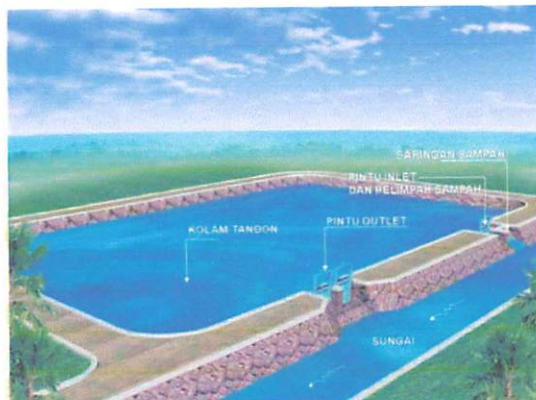
Gambar 6.12. Bangunan Pelimpah Samping ( Side Spillway )
