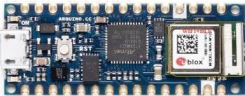
Gambar 7 Arduino Nano 33 IoT
