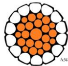
Gambar 2. 4 Locked Coil Ropes (STA-LOK, n.d)
