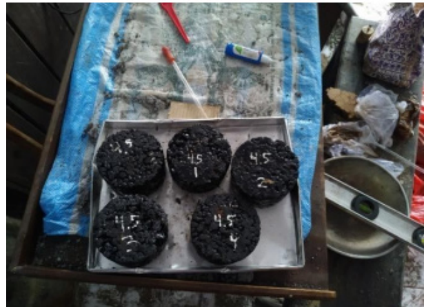
Figure 1. The Test Object of AC – WC Asphalt Briquette
