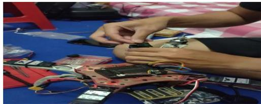
Gambar 3.8 Memasang *TX Reciver Transmitter* di *Flight Controller*
