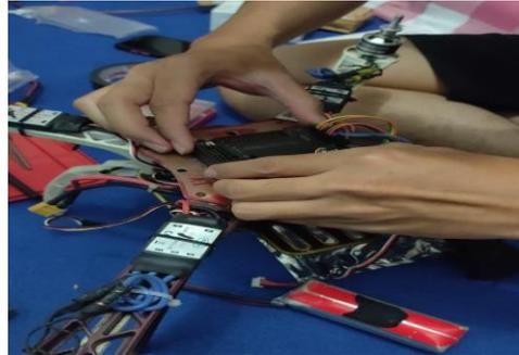
Gambar 3.6 Memasang *Flight Controller*
