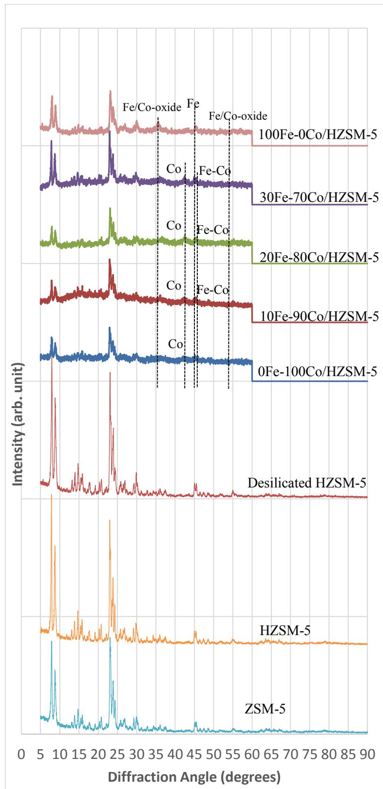
**Figure 2.** The XRD spectra for ZSM-5, HZSM-5, desilicated HZSM-5 and Fe-Co/HZSM-5 in various impregnation ratio after reduction by hydrogen at 400°C, 25 mL/min for 8 hours
