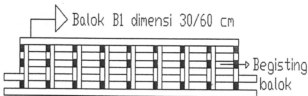
Gambar 4.6 Tampak samping begisting balok B1
