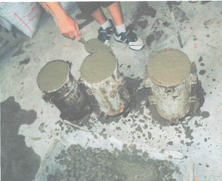
Benda uji Beton Normal
