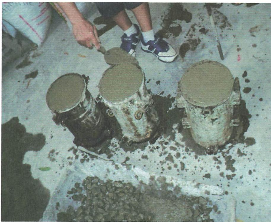
**Benda uji Beton Normal**
