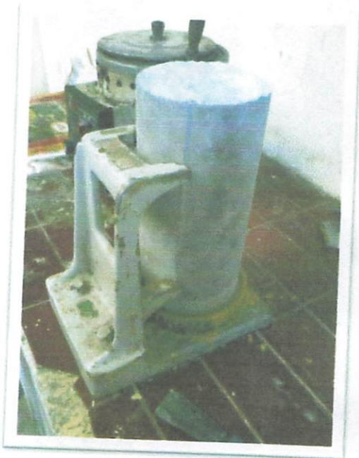
PROSES MEMBERI MORTAR BELERANG
