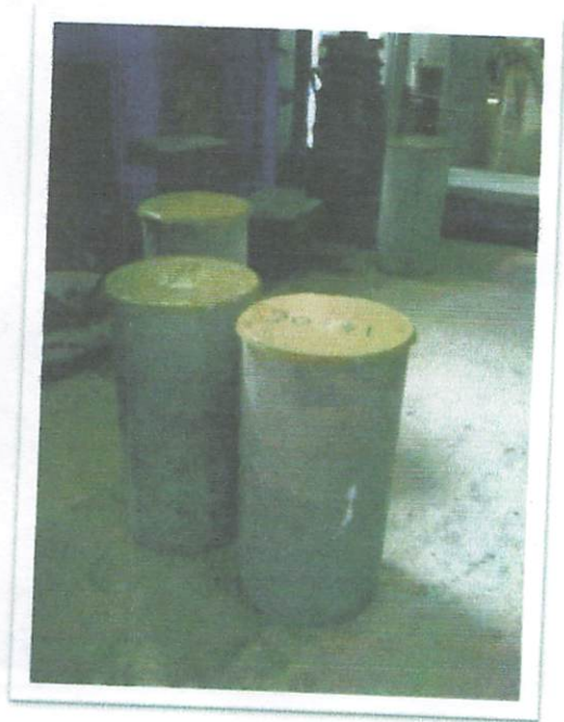
PROSES MEMBERI MORTAR BELERANG
