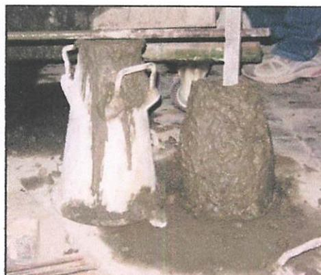
**Foto 1.2 : Pengukuran nilai slump = 86 mm**
