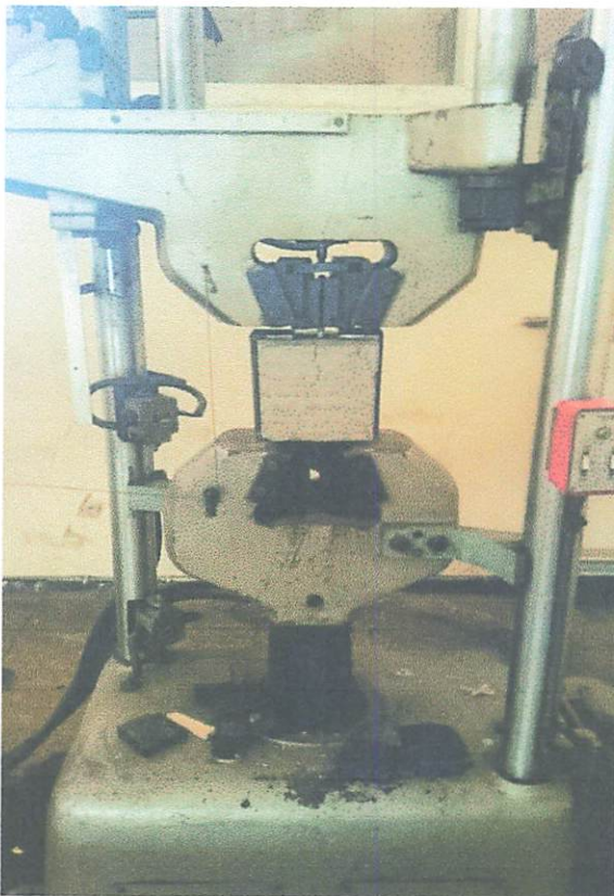
Gambar 4.8 : alat uji tarik Universal Testing Machine
