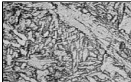
Gambar 2.4 Sementit Perbesaran 1000x (Sumber: ASM Handbook Volume 9 Metallography and Microstructure)
