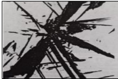
Gambar 2.7 Struktur Mikro Bainit Perbesaran 500x (Sumber: ASM Handbook Volume 9 Metallography And Microstructure)
