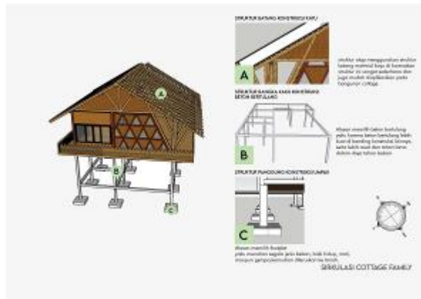
Gambar 9. Konsep Struktur Cottage tipe Family. Sumber : Analisa Pribadi,2023
