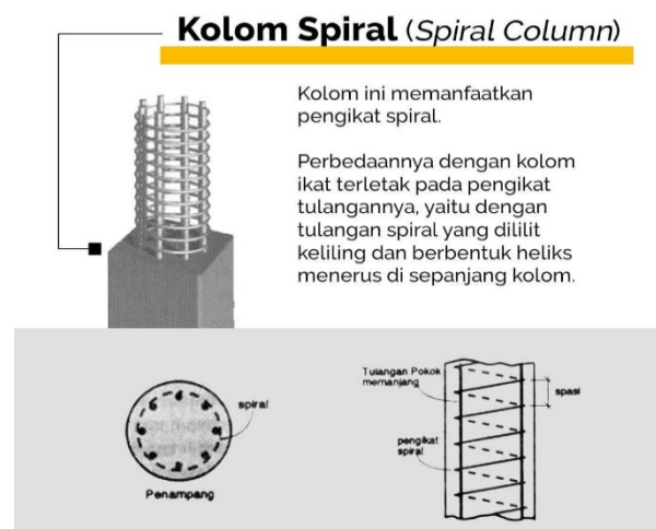
Gambar 69. Kolom Spiral
