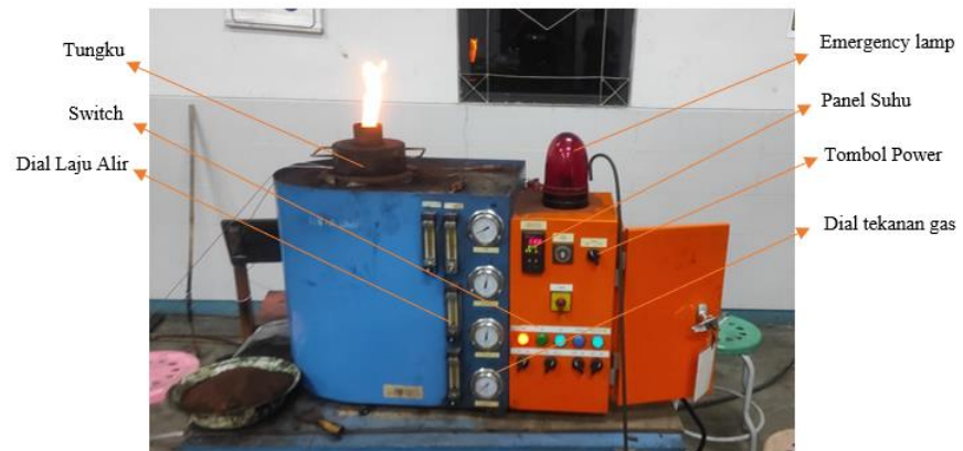
Gambar 3. 2 Fluidized Bed Furnace
