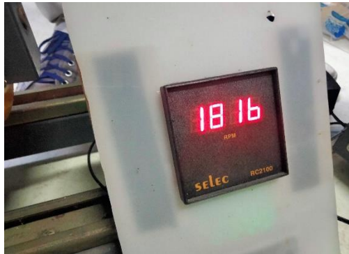
Gambar 4. 1 Hasil uji coba sensor proximity
