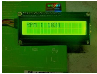
Gambar 11 Hasil uji coba sensor groove coupler
