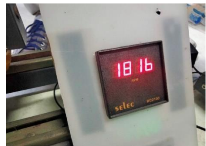
Gambar 10 Hasil uji coba sensor proximity
