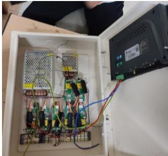
Gambar 21 Pengkoneksian Haiwell HMI SCADA
