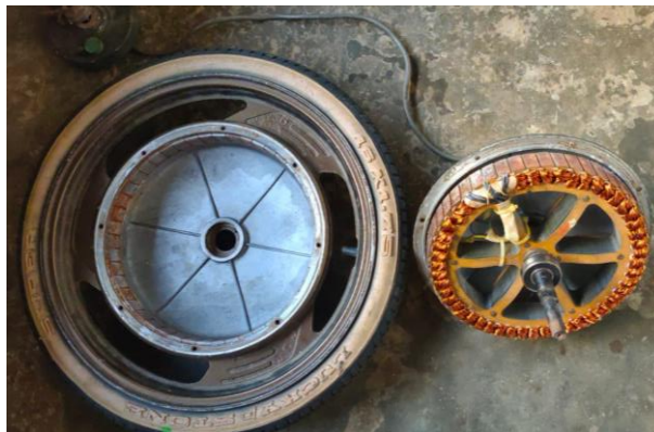
Gambar 4.5 Motor BLDC 48 V 500 Watt
