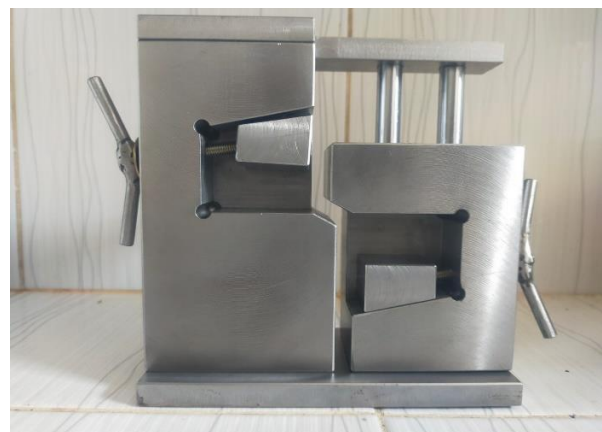
Gambar 10. Perakitan jig and fixture
