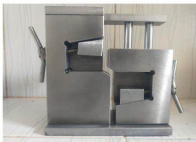
Gambar 10. Perakitan jig and fixture
