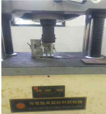
Gambar 11. Posisi Jig and Fixture di Universal Testing Machine (UTM)
