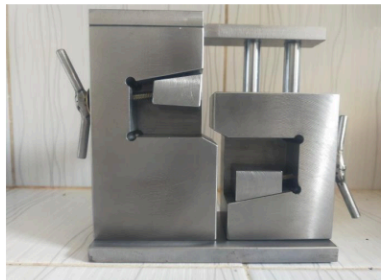
Gambar 10. Perakitan jig and fixture
