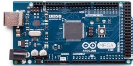
Gambar 5. Arduino Mega 2560
