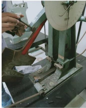
Gambar 3. 7 Impact Testing Machine
