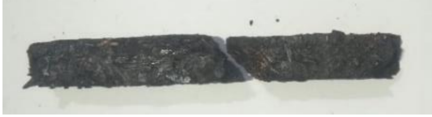
Gambar 15 : Hasil potongan uji impact charpy spesimen eco-paving block
