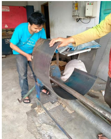
Gambar 4 : Proses bending plat 40 x 220 cm
