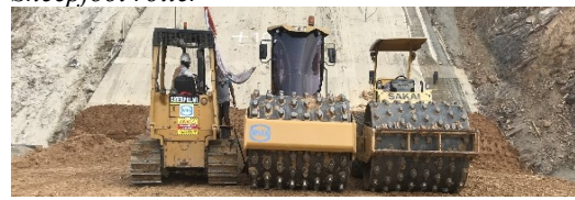
Gambar 5 Sheepfoot Roller CAT CS10 GC
