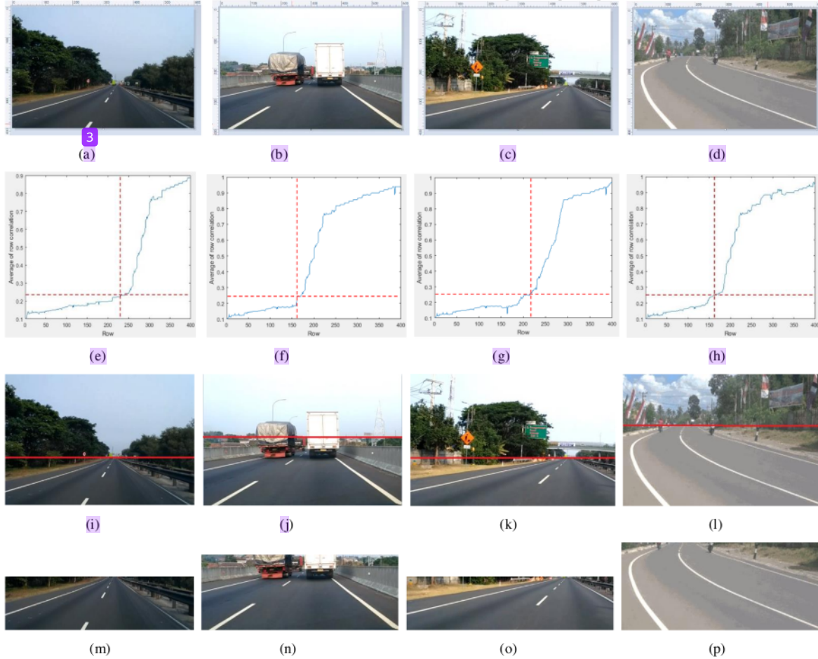
Figure 3. Pre-processing Result. (a) up to (d) are capturing image, (e) up to (h) are plotting of the row-correlation average, (i) up to (l) are the red line position, and (m) up to (p) are the result of road cutting.
