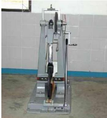
**Gambar 4.7 Alat Uji Impak**
