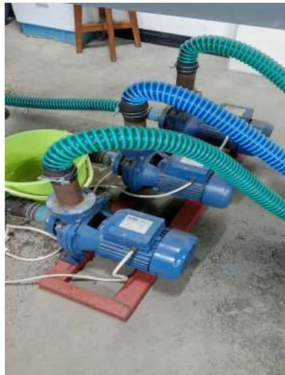
Gambar 3. Pompa Turbin Air Undershot
