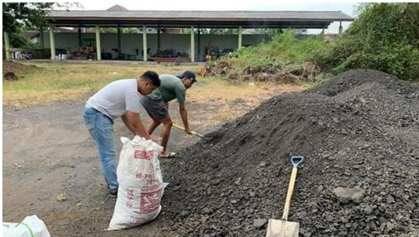
Gambar 2. 2 Limbah Aspal (Reclaimed Asphalt Pavement)
