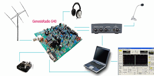
Gambar 2. Sistem Transceiver Genesis SDR [10]
