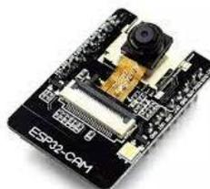
Gambar 2. ESP32-CAM
