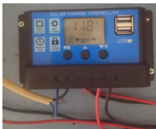
Gambar 4. 16 Solar Charger Controller
