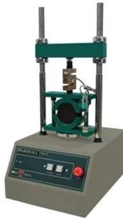
**Gambar 2. 9** Alat Uji Marshall
