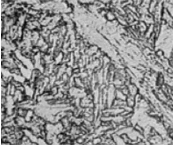
Gambar 2. 6 Sementit perbesaran 1000x ( Sumber : ASM Handbook Volume 9 Metallography and Microstructure )
