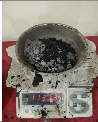
Gambar 18 Proses Penambahan Serbuk Ban
