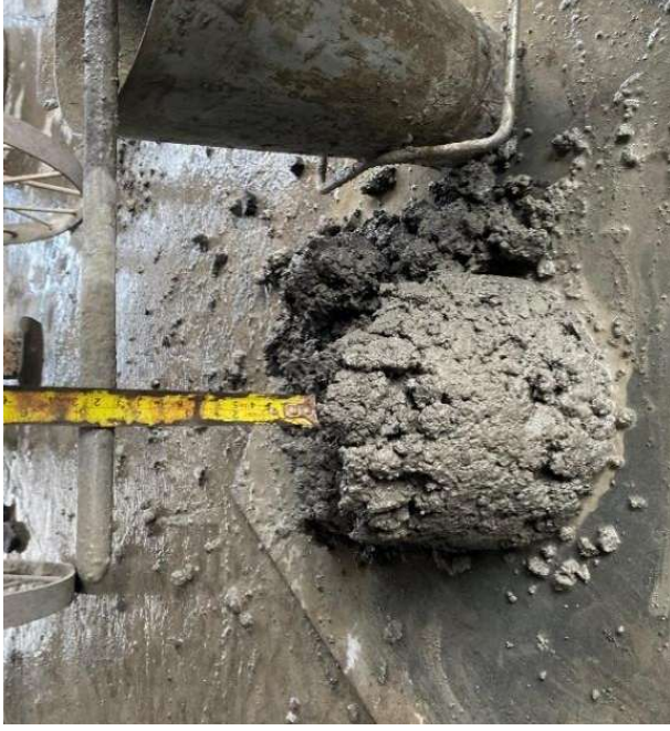
Gambar 4.23 Nilai Slump 12cm
