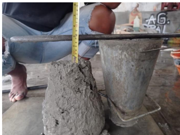
Gambar 4.16 Nilai slump 7 cm
