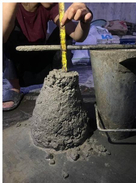
Gambar 4.18 Nilai slump 8 cm
