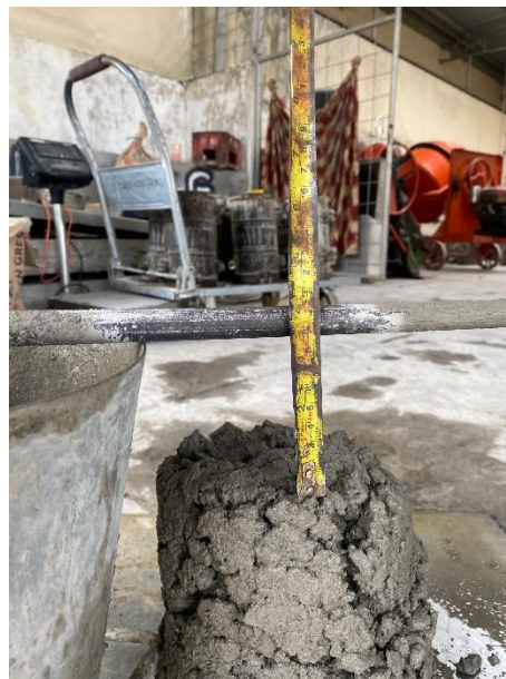
Gambar 4.20 Nilai slump 9,5 cm
