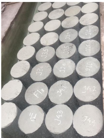
(Proses Curing Beton)
