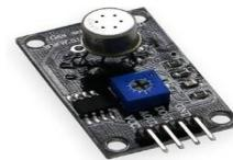
Gambar 9. Sensor TGS 2602
