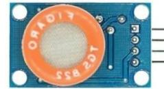
Gambar 7. Sensor TGS 822
