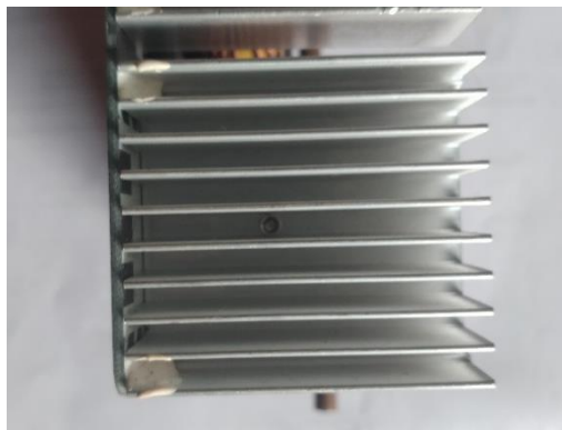
Gambar 3. 9 Heatsink (Sumber : Iqbal, 2024)
