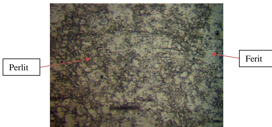
Gambar 4. 27 Hasil pengujian struktur mikro baja ST 37 treatment 2 menit U. Etsa: Nital 5%, alkohol 95%, perbesaran 500x
