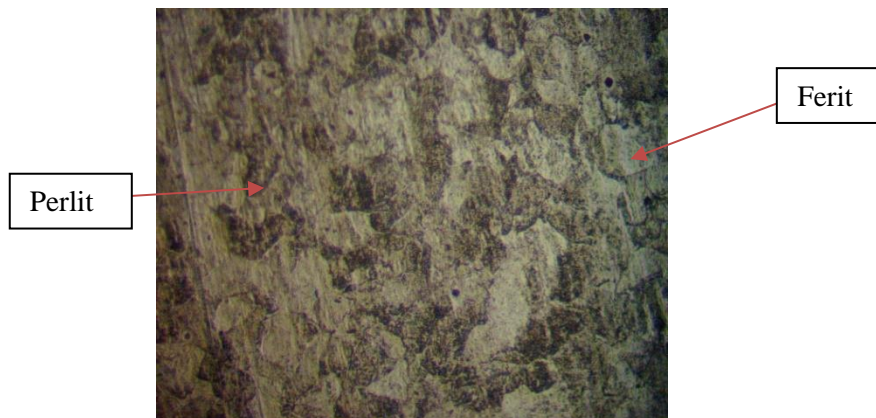
Gambar 4. 31 Hasil pengujian struktur mikro baja ST 37 treatment 3 menit Oval. Etsa: Nital 5%, alkohol 95%, perbesaran 500x
