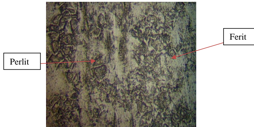
Gambar 4. 32 Hasil pengujian struktur mikro baja ST 37 treatment 4 menit Oval. Etsa: Nital 5%, alkohol 95%, perbesaran 500x
