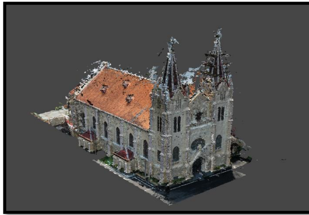
Gambar 3. 14 Proses Hasil Build Dense Cloud
