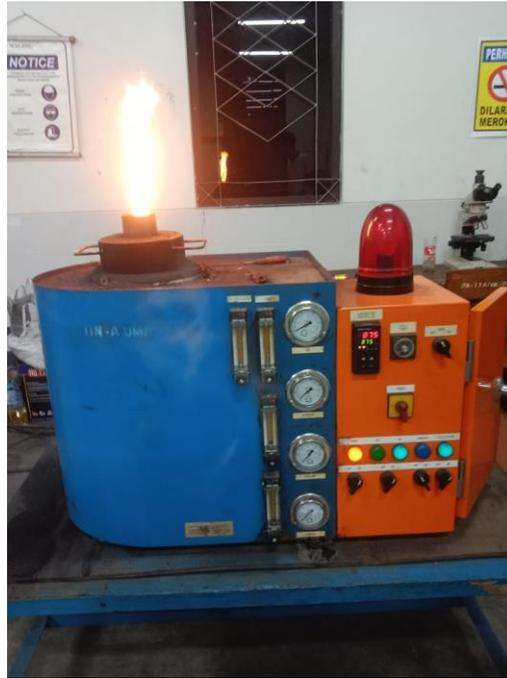
Gambar 3. 3 *Fluidized Bed Furnace*
