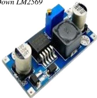
Gambar 4. Step Down LM2569
